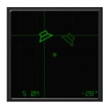
The **Elev** CV input will offset the elevation of the audio source.
